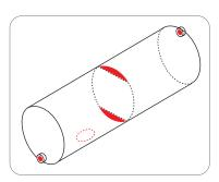
It should be possible to view the interior of the vessel through either the vent holes or an inspection hole. Holes/ Lugs must be provided so the fabrication may be hung by wires onto jigs.
