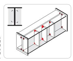
External Stiffners on open sections should incorporate cropped corners or drainage holes to eliminate dead pockets.
