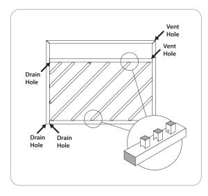
✓ If drain holes are too small, the zinc will not be able to enter quickly enough and the item may be become buoyant causing it to float off the jig or be subject to erratic immersion.
